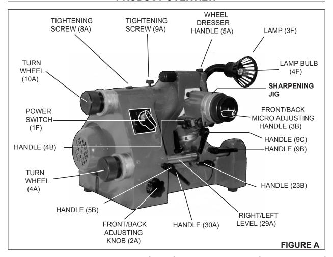
Prior to operating the Universal Cutter/Grinder, make sure you familiarize yourself with the main parts components and their functions. (See Figure A, and Assy. Diagrams A, B, C, and F.)
